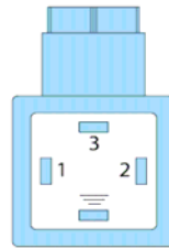
4 Pin Hirschmann style mating-half & Pin information
