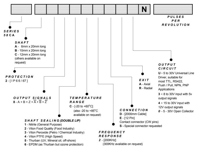
Note: All shaft seals are double-lip and are fitted with appropriate grease.
